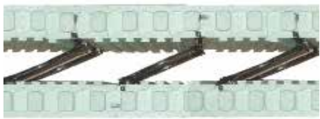
Close view of folding metal-hinged web
